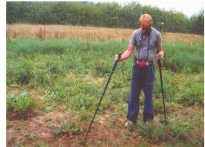
In order to determine various characteristics about a fault, such as severity, shape, corrosion behaviour, etc, various electrical measurements around the epicentre and from epicentre to earth are made for interpretation.
