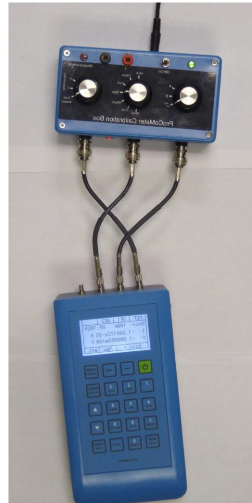
ProCoMeter Connected to the Calibration Box
