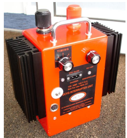
125amp Satellite Synchronised Interrupter
